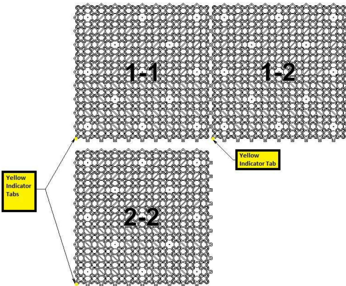
2. Install the AirPave panels across the field in a rowed pattern. Staggering of rows will allow for multiple row completion by a multi-manned crew.
