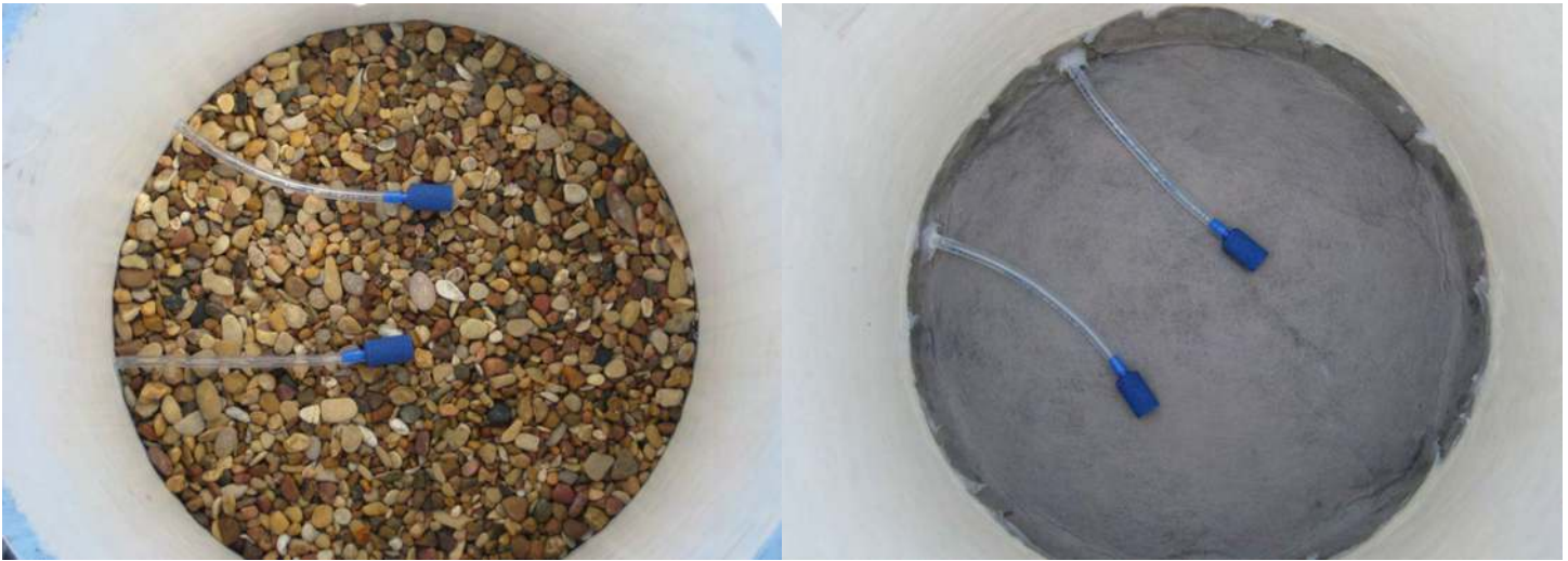
Figure 3. Test greens constructed in 14-inch PVC pipe with either gravel or geotextile atop AirDrain as the drainage layers. Both types of test greens contained a pair of porous cups connected to plastic tubing that formed manometer–tensiometers to allow measurement of water pressure or tension at the root zone–drainage layer interface.
