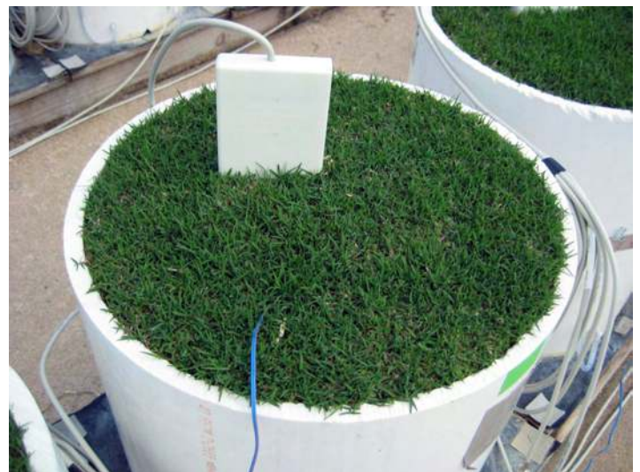
Figure 4. Test green with vertically installed, 1–ft long TDR probe used to measure average water content within the root zone profile.
