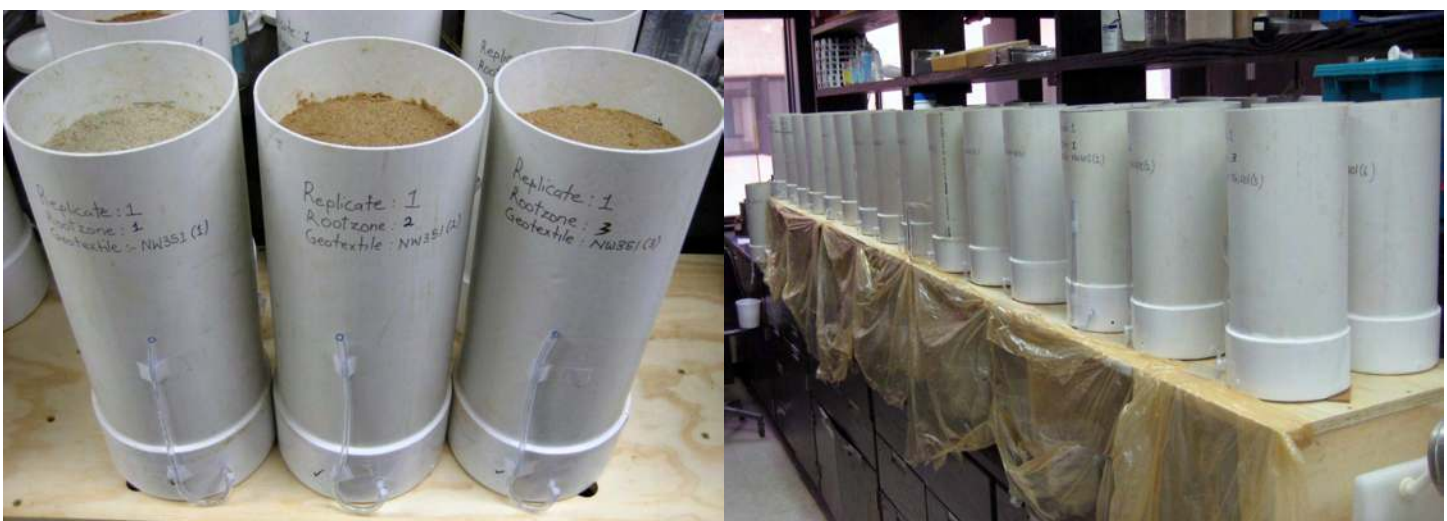
Figure 6. Columns used to measure potential clogging of geotextiles by fines migrating out of the root zone.
