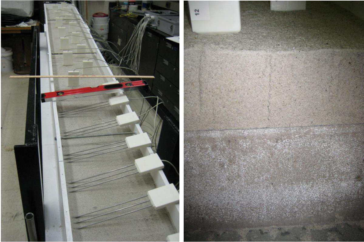
Figure 14. Sloping test box with TDR water content probes (left) and excavated section showing subsurface clear plastic barrier in place at the bottom of the root zone profile (right).
